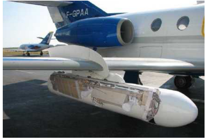
Fig. 4. Cutaway view of a SETHI pod.
