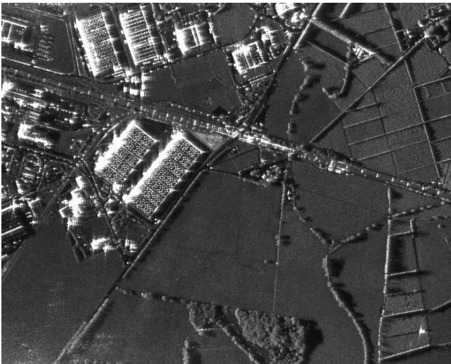
Fig. 13. Monostatic SAR image of the same scene (remark the important specular reflections on the building edges).
