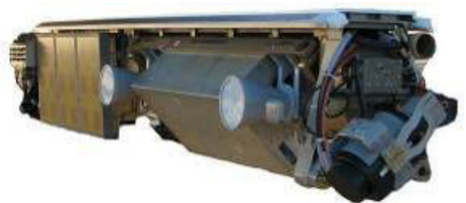
Fig. 5. X + L bands and visible-band camera configuration.
