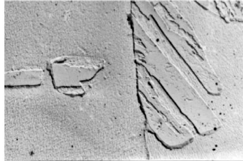
Fig. 4. Nucleation of austenite at ferrite grain boundaries in the 10HSND grade steel: (a) 1000x, (b) 4800x [8]
