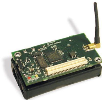
Fig. 1. MICAz mote for which the idea is proposed. These motes lose their battery voltage with the passage of time.
