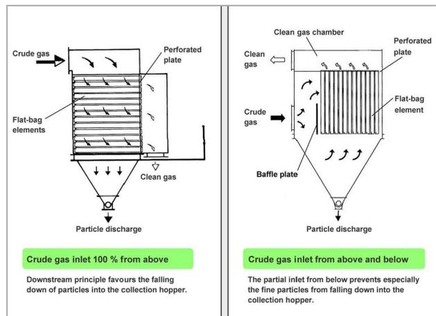
Fig. 7. Gas flow to the filter elements
