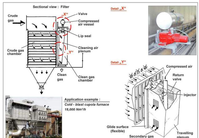
Fig. 4. Travelling compressed air – off line – cleaning
