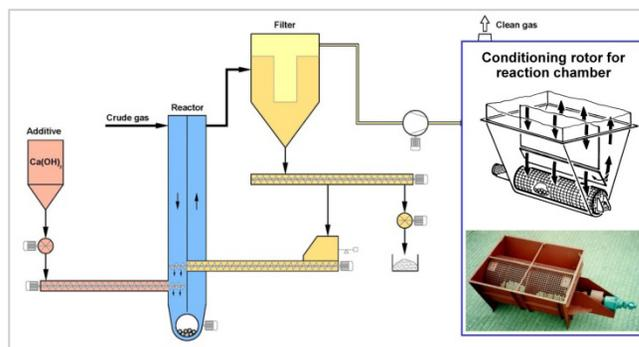
Fig. 9. Conditioning Rotor – Recycle Process (KUV)
