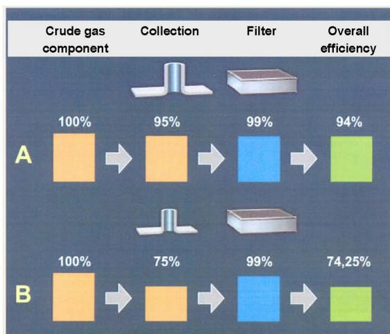
Fig. 1. Influence of collection system on the overall efficiency [2]
