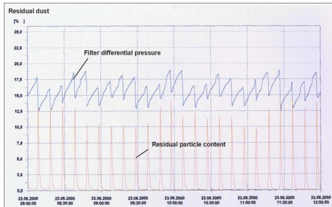
Fig. 6. Influence of the cleaning cycle on the residual particle content in the clean gas
