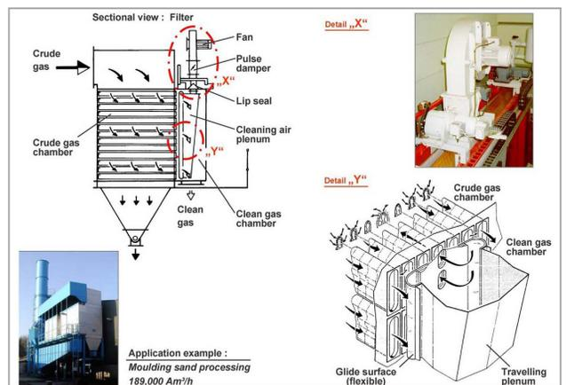
Fig. 5. Travelling medium pressure – off line – cleaning
