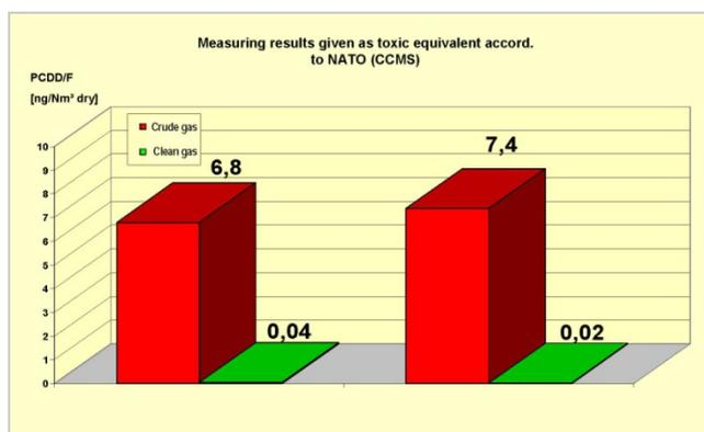
Fig. 10. Dioxin/ Furan separation from the off-gas of melting furnaces for secondary aluminium
