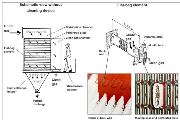
Fig. 3. Schematic view of flat-bag filter and filter element – horizontal installation
