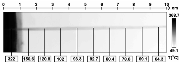
Fig. 1. Distribution of temperature in wire after deformation, obtained by the infrared camera
