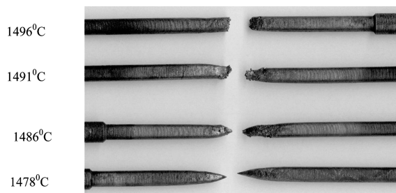
Fig. 1. Samples of cast carbon steel (0,22%C) after testing at different temperatures
