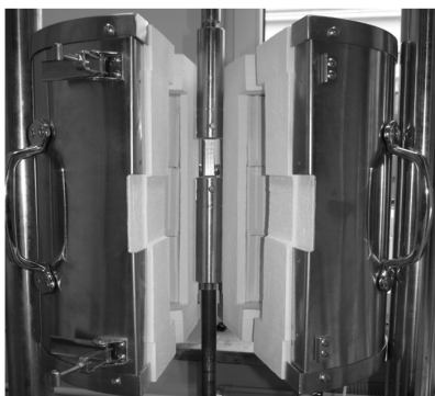
Fig. 4. Stress rupture test stand
