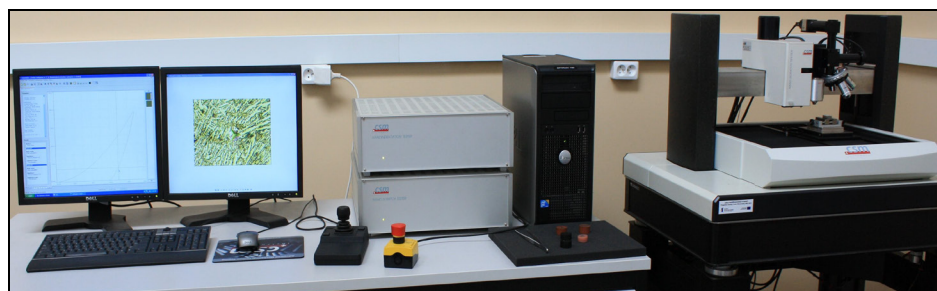
Fig. 2. The test method for indentation testing, OPX NHT / NST's CSM Instruments
