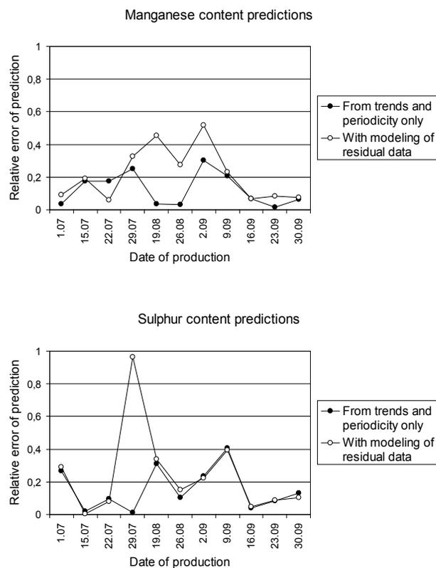
Fig. 5. Comparison of prediction errors for Mn and S contents in cast iron, for the first measurements recorded after 12 am, on Wednesdays, during three months
