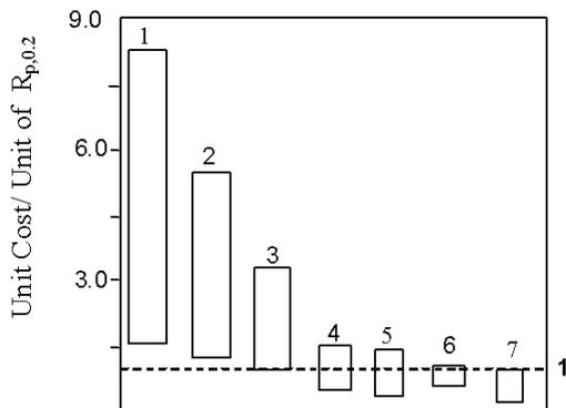
Fig. 2. Unit costs<sup>1</sup> of product essential for obtaining unit yield strength  $R_{p0.2}$  normalized towards forged steel (up to 1); (1) - aluminum alloys castings, (2) - forged aluminum, (3) - cast steel, (4) - forged steel, (5) - heat treated steel, (6) - ductile iron, (7) - ADI [1]
