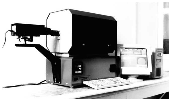
Fig. 1. A high-temperature microscope applied in the measurements of liquid Cu-Ag alloy surface tension
