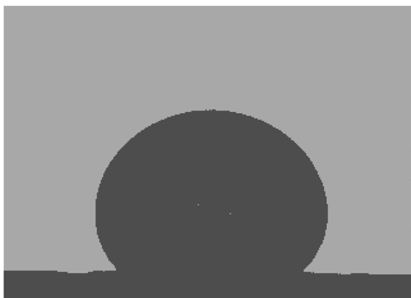
Fig. 2. A drop of the Cu-10% mass Ag on an \text{Al}_2\text{O}_3 plate at 1473 K, recorded during the investigations
