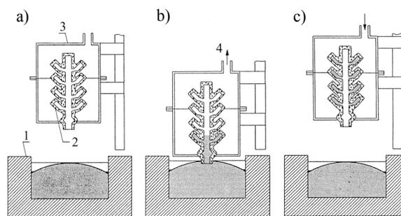
Fig. 2. The principle of operation of a method using back-pressure for filling of investment moulds:
