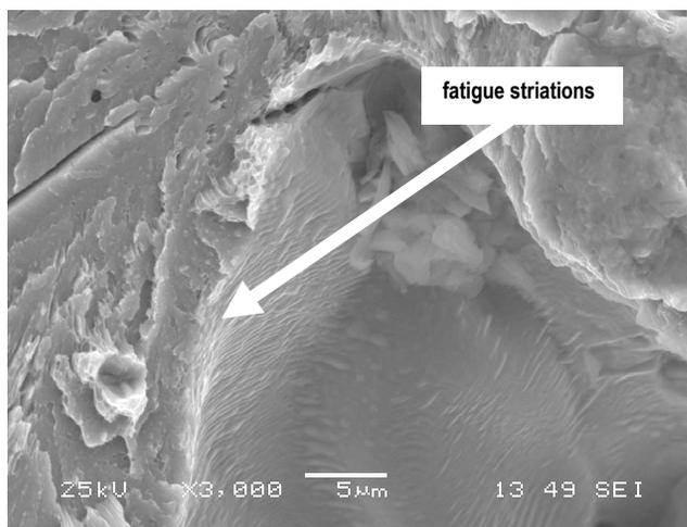
Ductile iron. Specimen 3, x3000, SEM.
