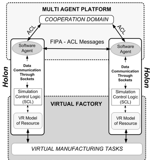
Fig. 2. The architecture of virtual holonic factory. Source: [1]
