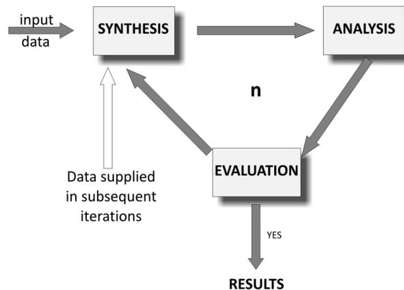
Fig. 3. Iterative loop in design
