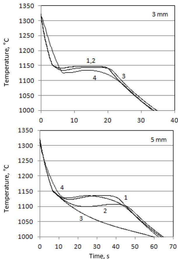
Fig. 1. Fragments of the casting cooling curves. The results of simulation obtained for the following eutectic grain densities: casting wall thickness: 3 mm: 1 -  $n=10^{15}$ , 2 -  $n=9.7 \cdot 10^{14}$ , 3 -  $n=5 \cdot 10^{14}$  m<sup>-3</sup>; casting wall thickness: 5 mm: 1 -  $n=10^{14}$ , 2 -  $n=3.8 \cdot 10^{13}$ , 3 -  $10^{13}$  m<sup>-3</sup>, 4 – the result of measurement.
