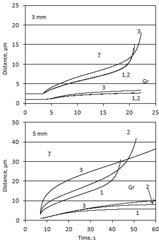
Fig. 2. Changes in the position of „graphite-austenite” (Gr) and „austenite-liquid” ( $\gamma$ ) phase boundaries in castings with the wall thickness of 3 mm (the densities of eutectic grains: 1 -  $n=10^{15}$ , 2 -  $n=9.7 \cdot 10^{14}$ , 3 -  $n=5 \cdot 10^{14} \text{ m}^{-3}$ ) and 5 mm (the densities of eutectic grains: 1 -  $n=10^{14}$ , 2 -  $n=3.8 \cdot 10^{13}$ , 3 -  $10^{13} \text{ m}^{-3}$ ) – the results of simulation
