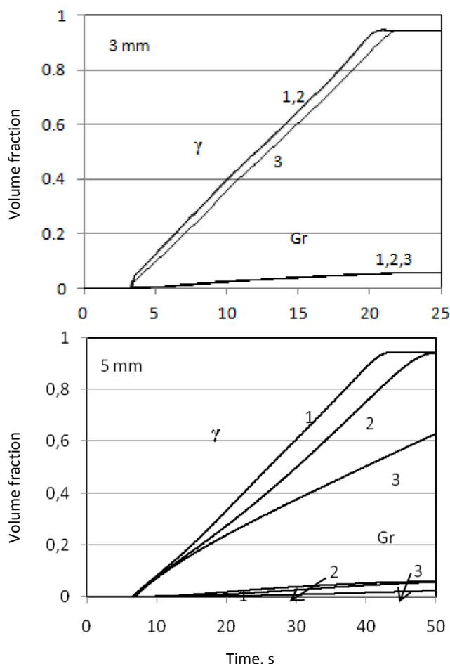
Fig. 3. Changes in the volume fraction of graphite (Gr) and austenite ( $\gamma$ ) in castings with the wall thickness of 3 mm (the densities of eutectic grains: 1 -  $n=10^{15}$ , 2 -  $n=9.7 \cdot 10^{14}$ , 3 -  $n=5 \cdot 10^{14} \text{ m}^{-3}$ ) and 5 mm (the densities of eutectic grains: 1 -  $n=10^{14}$ , 2 -  $n=3.8 \cdot 10^{13}$ , 3 -  $10^{13} \text{ m}^{-3}$ ) – the results of simulation
