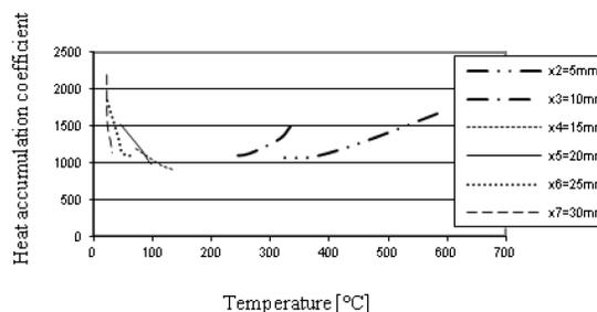
Fig. 4. The temperature dependence of the heat accumulation coefficient of the moulding sand O.B.B. Sand 'E'
