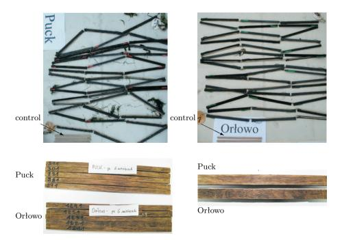
Fig. 2. The wood samples after remaining immersed in the Baltic Sea for 6 months
