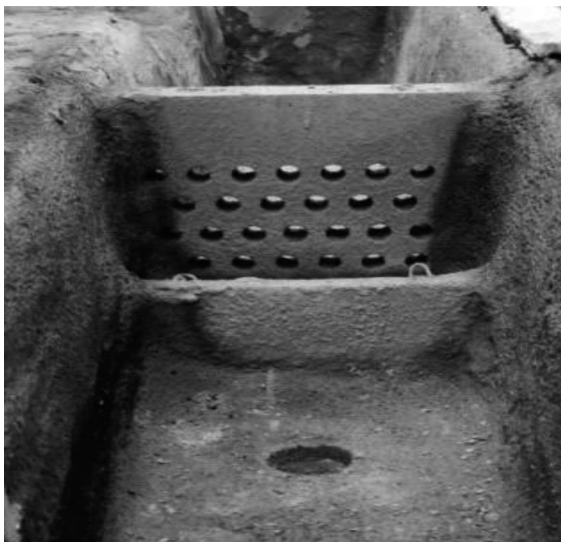
Fig. 3. Tundish of the CC machine provided with the ceramic filter
