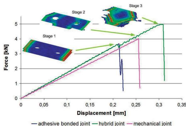
Fig. 6. Stages of deformation of the analysed joints
