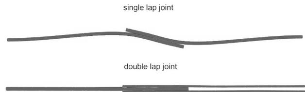
Fig. 7. Joints deformation
