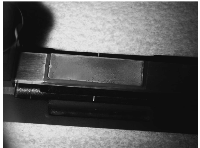
Fig. 3. Distribution of isochromatics in the sample of optically active layer
