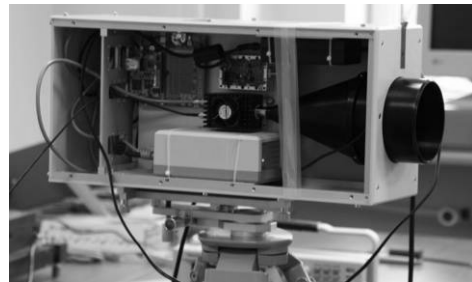
Fig. 11. Photo of the FSO transmitter (a) and the FSO receiver (b) (2 nd generation) [11]
