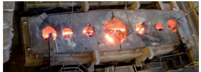
Fig. 13. Ladle with the innovatory cover after finished cycle of pourings
