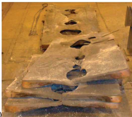
Fig. 8. Side cover made of 25 mm sheet, strengthened by transverse and longitudinal shaped elements, shown without its refractory lining, and worn covers
