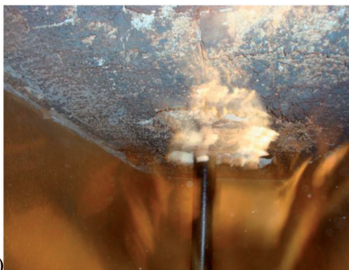
Fig. 12. Insulating material of the cover after a certain exploitation period – a) Magnified fragment of the cover after a much longer exploitation – b)
