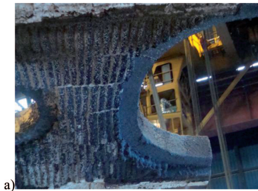
Fig. 11. Cover during heating and filling with liquid steel. White edges of insulated holes indicate that a temperature exceeded 900°C
