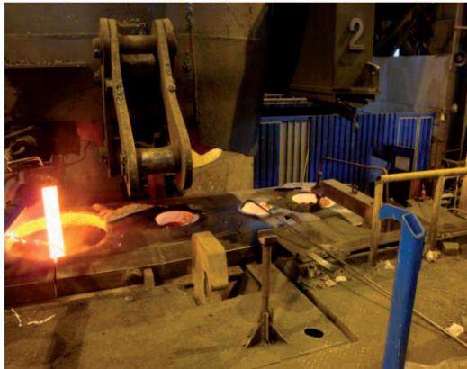
Fig. 11. Cover during heating and filling with liquid steel. White edges of insulated holes indicate that a temperature exceeded 900°C
