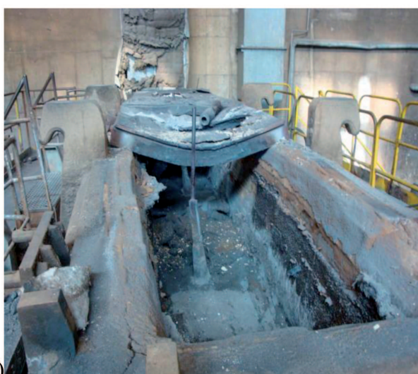
Fig. 4. Examples of thermal deformations of the tundish cover [4]
