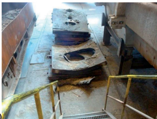
Fig. 7. New and worn middle part of the cover with the largest hole
