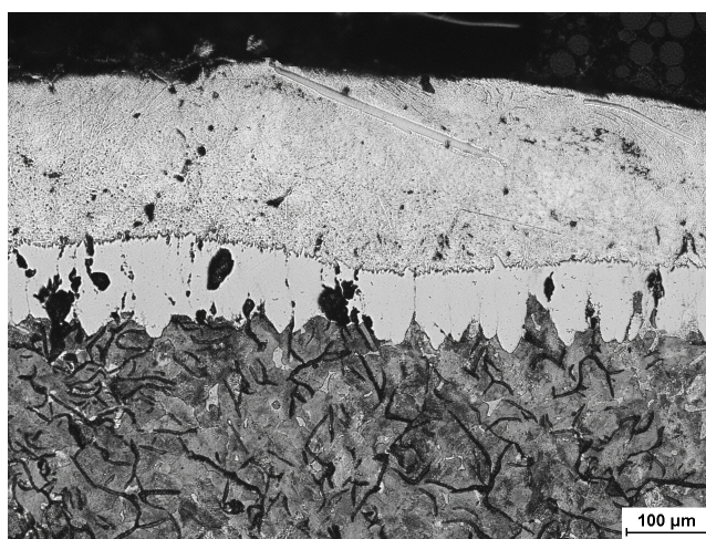
Fig. 8. An optical micrograph of graphite cast iron hot-dip coated with AlTi5 alloy
