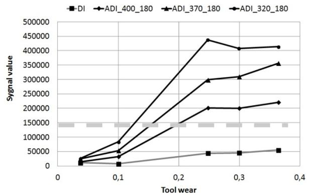
Fig. 7. Signal of vibration –Vz mom2 for different DI samples
