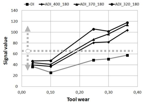
Fig. 4. Signal of cutting force  $-F_z$  in the 2<sup>nd</sup> second of cutting for different DI samples
