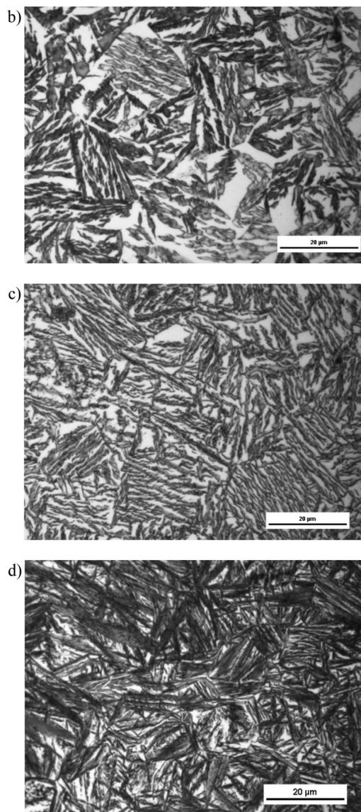
Fig. 1. Microstructure of ductile iron samples;
