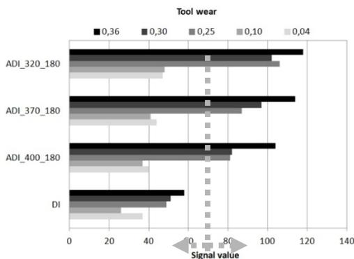
Fig. 3. Signal of cutting force  $-F_z$  in the 2<sup>nd</sup> second of cutting for different DI samples
