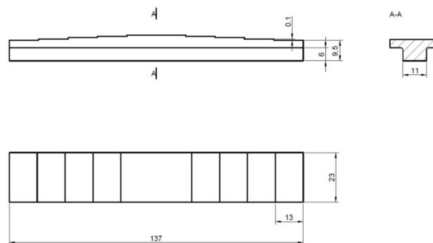
Fig. 2. Pictorial drawing of the sample
