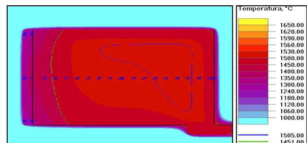
Fig. 9. Temperature distribution after 45 s; cuboid 80x80x100[mm]; pouring temperature 1510°C
