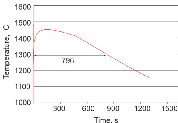
Fig. 5. The curve of temperature changes in time; thermocouple pad; cuboid 90x90x80mm (pouring temperature 1550°C)
