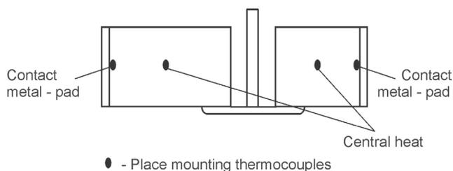
Fig. 3. Arrangement of the thermoelements
