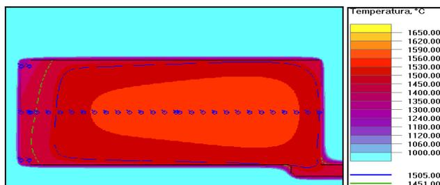
Fig. 7. Temperature distribution after 45 s; cuboid 70x70x150[mm]; pouring temperature 1600°C
