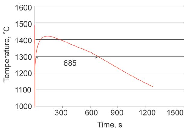
Fig. 6. The curve of temperature changes in time; thermocouple pad; cuboid 80x80x100mm (pouring temperature 1510°C)
