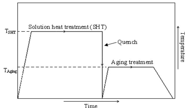
Fig. 1. Heat treatment of alloy
