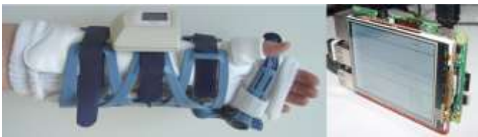
Fig. 5: Depiction of measurement system and portable Linux based embedded system
