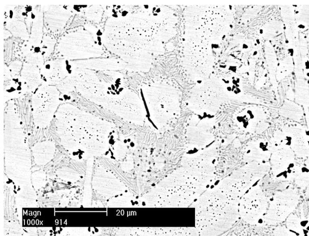
Fig. 9. The shape and location of the  $\kappa$ -phase precipitates in the microstructure of BA1055 bronze castings, (SEM)
