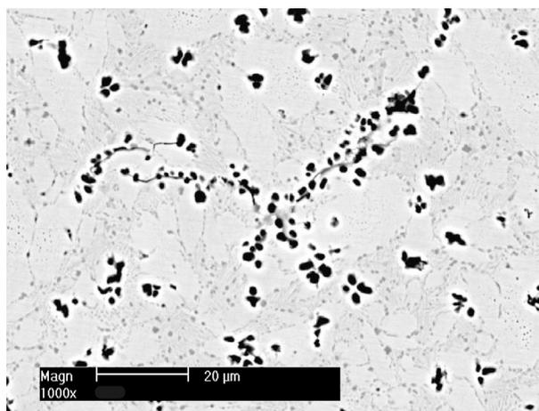
Fig. 10. The shape and location of the  $\kappa$ -phase precipitates in the microstructure of BA1055 bronze castings, (SEM)
