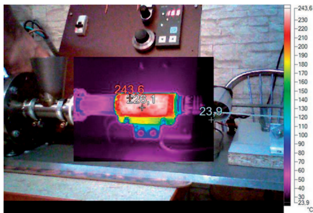
Fig. 3. Extruder visible in FLIR thermal imager
