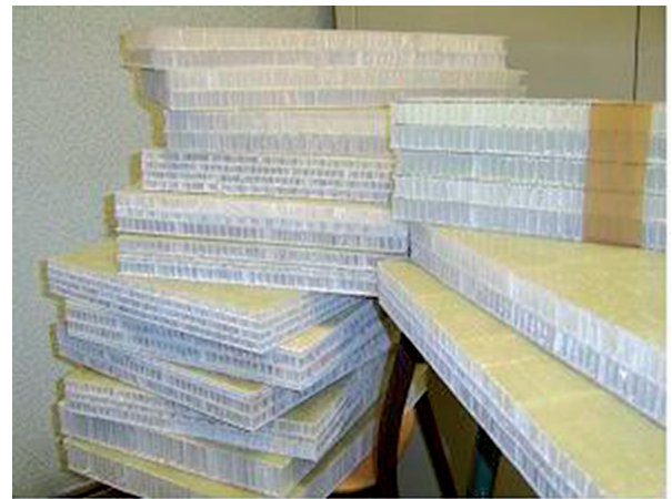
Fig. 3. Honeycomb multi-layer sandwich
