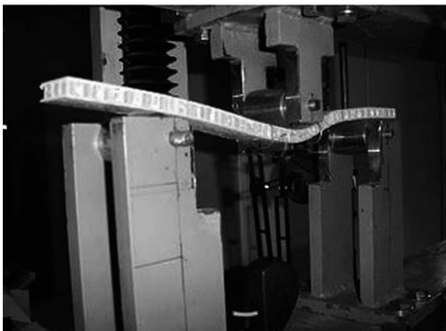
Fig. 4. Three-points bending test
