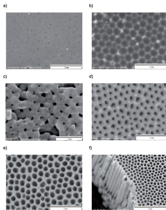
Fig. 5. SEM images of the membrane after each of the process stage: a – after the first stage of anodizing, b – after the removal of Al<sub>2</sub>O<sub>3</sub>, c – after the second stage of anodizing, d – after the widening of pores e – after the removal of the barrier film f – the membrane prepared for cathodic deposition of Co-Fe nanowires
