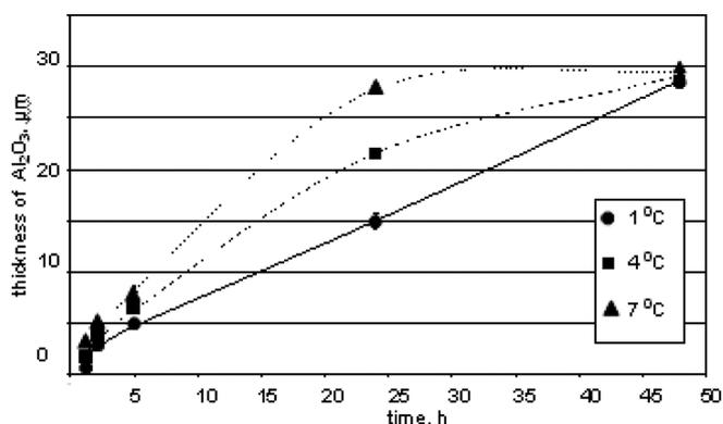
Fig. 1. The relationship between the thickness of the oxide film and anodizing time and temperature
