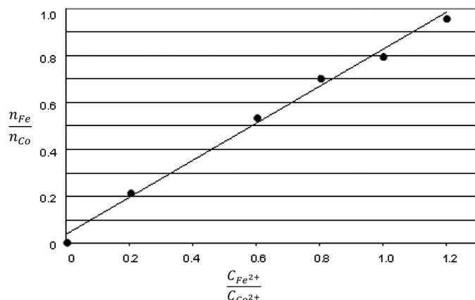
Fig. 7. The relationship between the ratio of the number of moles ( $n_{Fe} / n_{Co}$ ) of both metals in the cathodic deposit (Co-Fe alloy) and the ratio of the concentrations of ions ( $C_{Fe^{2+}} / C_{Co^{2+}}$ ) in the electrolyte
