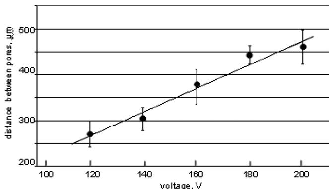
Fig. 3. The relationship between the distance between pores and the electrolysis voltage; anodizing conditions: 0.17 M H<sub>3</sub>PO<sub>4</sub> solution, time 24 h, temperature 1°C
