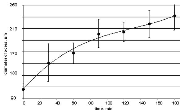
Fig. 4. The influence of the chemical treatment time on the diameters of pores in Al<sub>2</sub>O<sub>3</sub> membranes; anodizing conditions: 0.17 M H<sub>3</sub>PO<sub>4</sub> solution, temperature 1°C, the voltage 180 V
