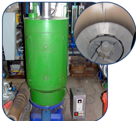
Fig. 1. Fragment of the experimental rotor mechanical reclaimer RD-6 with an internal system of grinding elements
