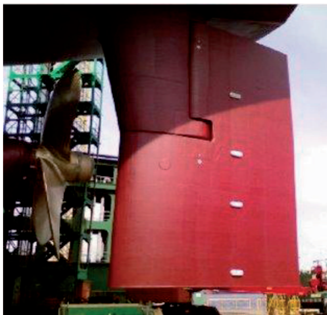
Fig. 1. The arrangement of protectors on ship's flap rudder
