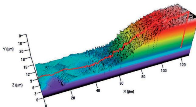
Fig. 4. Three-dimensional surface topography (CLSM) of the front electrode prepared from the PV 145 paste on a surface without texture and with antireflection layer co-fired in the furnace at  $830^{\circ}\text{C}$  temperature (example)
