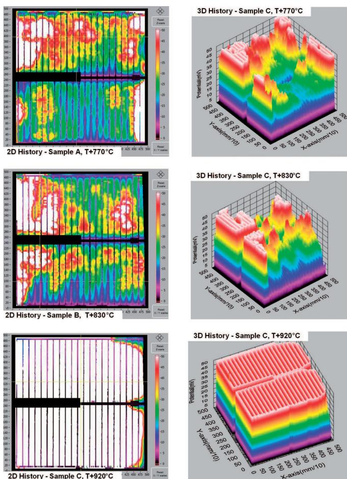
Fig. 5. Corescan potential mappings on cells co-fired at various temperature. Lighter areas have higher contact resistance
