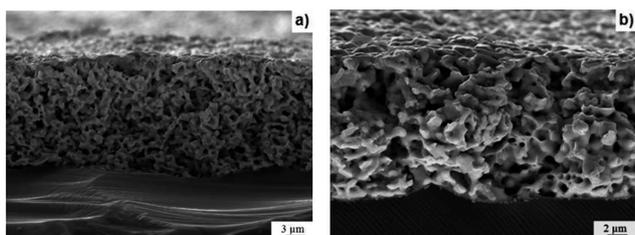
Fig. 3. SEM fracture images of front contact layer co-fired in the furnace at the temperature: a)  $770^{\circ}\text{C}$ , b)  $920^{\circ}\text{C}$  from PV 145 paste on Si substrate without texture and with antireflection layer
