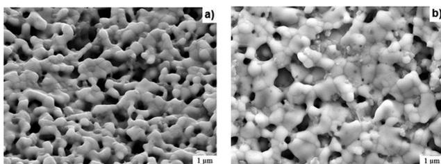
Fig. 2. SEM images of front contact layer co-fired in the furnace at the temperature: a)  $770^{\circ}\text{C}$ , b)  $920^{\circ}\text{C}$  from PV 145 paste on Si substrate without texture and with antireflection layer
