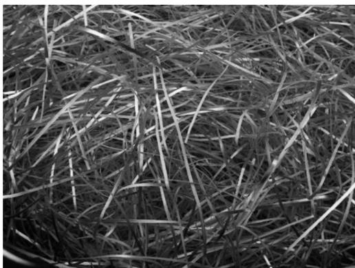
Fig. 7. The appearance of RS ribbon cast from AZ91 alloy
