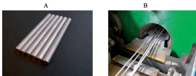
Fig. 5. A, B – Hot extrusion product
