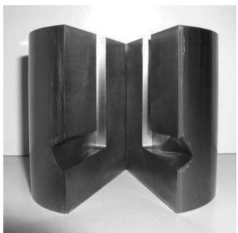
Fig. 5. ECAP tool with helix matrix
