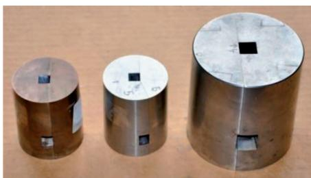
Fig. 6. General view on used ECAP tools
