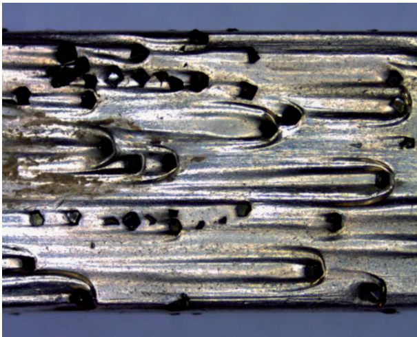
Fig. 2. Diamond grits retained on a working surface of a segment
