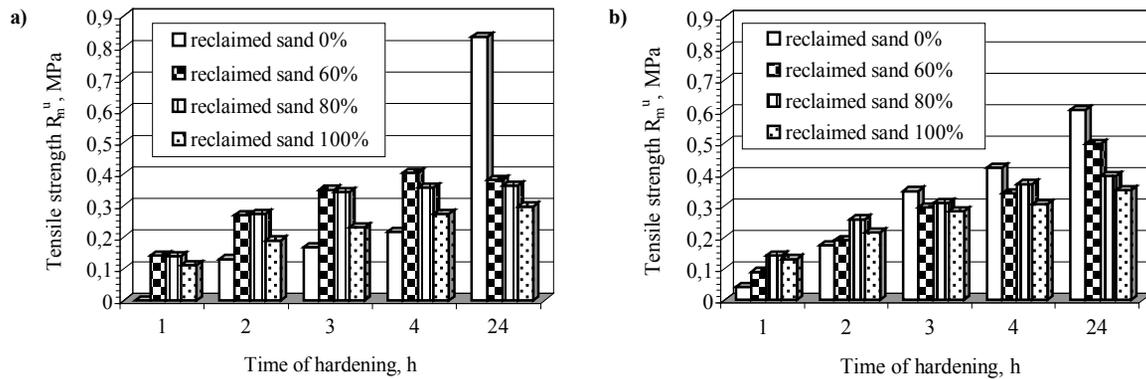
Fig. 1. Influence of the hardening time on the tensile strength,  $R_m^u$  of the moulding sand of the composition: high-silica sand 0 – 100 parts by mass, reclaim 0 – 100 parts by mass, GEOPOL binder 2.0 parts by mass, hardener – 14% of the binder amount: a) SA72, b) KR72
