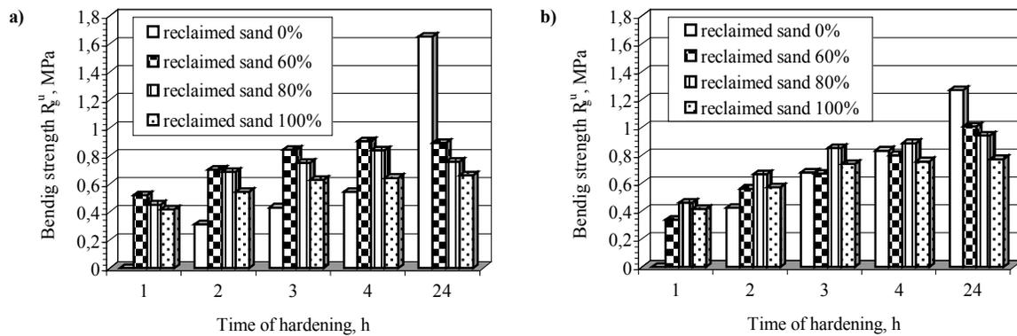
Fig. 2. Influence of the hardening time on the bending strength,  $R_g^u$  of the moulding sand of the composition: high-silica sand 0 – 100 parts by mass, reclaim 0 – 100 parts by mass, GEOPOL binder 2.0 parts by mass, hardener – 14% of the binder amount: a) SA72, b) KR72
