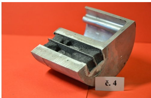
Fig. 6. H 2400 during dissolution of the glued core
