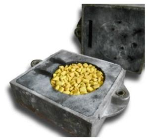
Fig. 3. Mold filled with precursors
