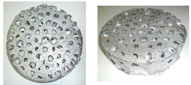
Fig. 9. Casting (AlSi10MgMn) – type II
