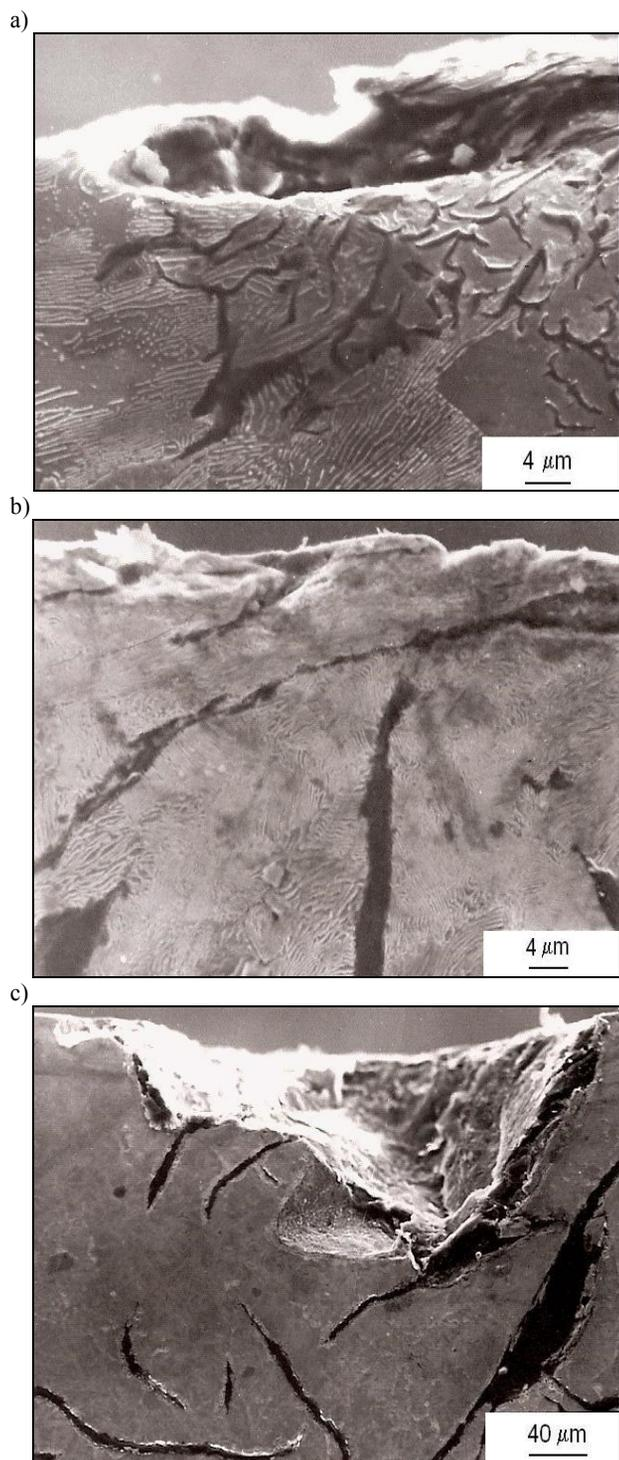
Fig. 1. Cylinder liner material wear with a diversified morphology of flake graphite precipitations. Visible are material tear-outs in the area of fine graphite precipitations sites with sizes of up to 15  $\mu\text{m}$  and interdendritic distribution; (a) a view of the load bearing surface; (b), (c) views in the plane perpendicular to the bearing surface
