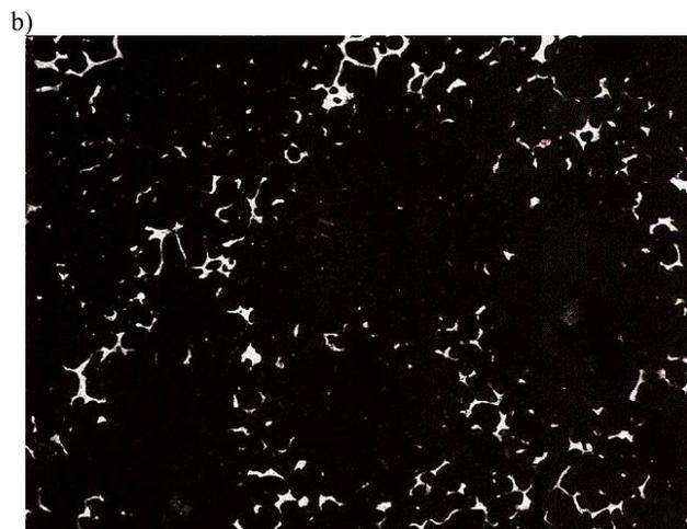
Fig. 6. Distribution of phosphide eutectic in the experimental liner casting: (a) in the area adjacent to the inner surface and (b) at half thickness of the casting wall. Etching in 4% HNO<sub>3</sub>. Magnification 50×.
