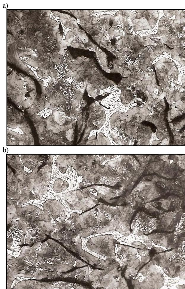
Fig. 5. Structure of the experimental liner casting: (a) in the area adjacent to the inner surface and (b) at half thickness of the casting wall. Etching in 4% HNO<sub>3</sub>. Magnification 250 $\times$
