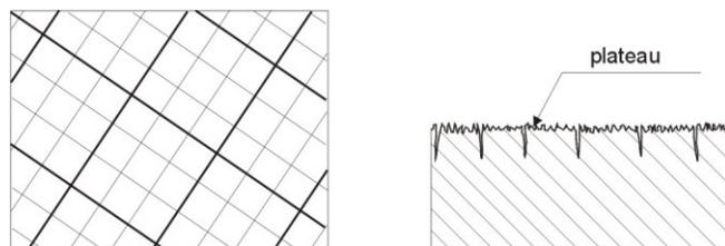
Fig. 2. Schematic diagram of a surface honed to shape a plateau
