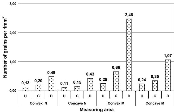
Fig. 7. Number of grains per 1mm<sup>2</sup> in dependence on the surface type and measuring area
