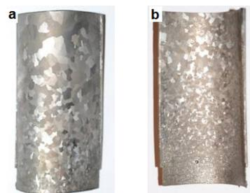
Fig. 3. Casting macrostructure: a) convex surface (1) – unmodified, b) concave surface (2) - modified
