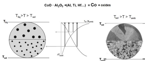
Fig. 11. The effect of undercooling on the nucleation process and macrostructure of the IN-713C alloy casting obtained using mould with modifying surface [7]
