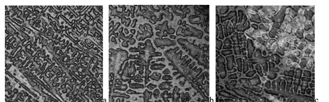
Fig. 7. CuSn8Ni bronze ingot micro-structure, cast into a metal mould before modification (a), after modification with Kupmod Z formula in the amount of 0.2% (b) and 0.3% of the metal stock weight (c). Magnification 300x, etched with a mixture of acids
