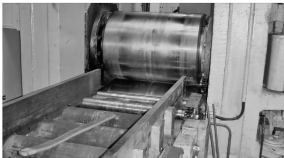
Fig. 4. View of cold rolling process of \phi 30 mm Al continuous ingot to 5 mm thick flat
