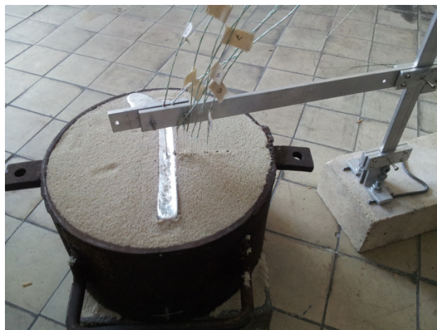
Fig. 2. The experimental mould after pouring. Visible thermocouples mounted in the mould cavity and in the mould body [9, 12]
