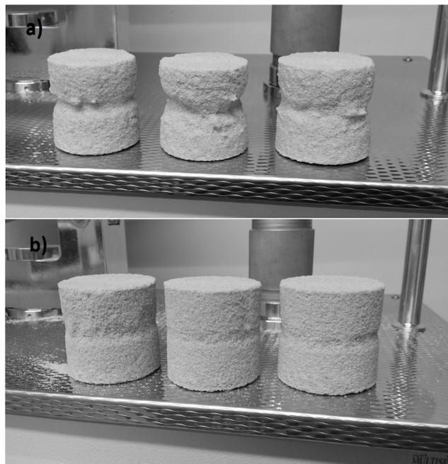
Fig. 6. Traditionally dried specimens after abrasion wear test, prepared in variant 0% (a) and in variant 1% (b)
