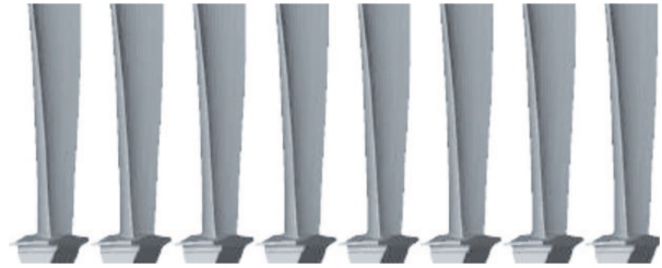
Fig. 6. *.CAD model of pattern assembly
