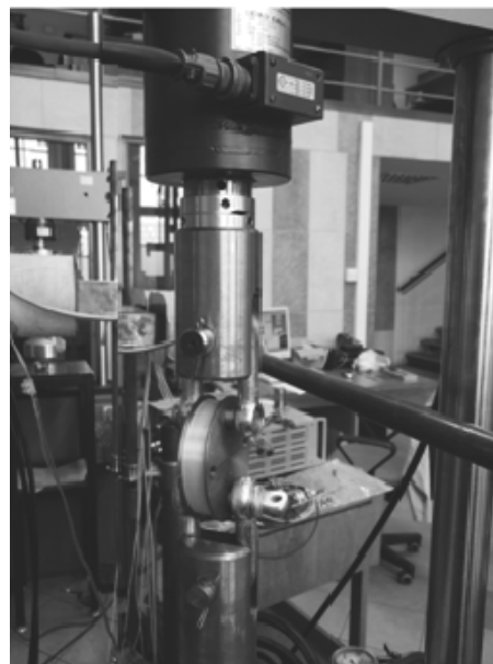
Fig. 1. The aramid-silicone composite materials in the tests with the non-standard NOL rings and hydraulic pulsator MTS 810 use; a) the type of non-standard NOL tooling of wound aramid fibre; b) sample installed in the grips of the testing machine
