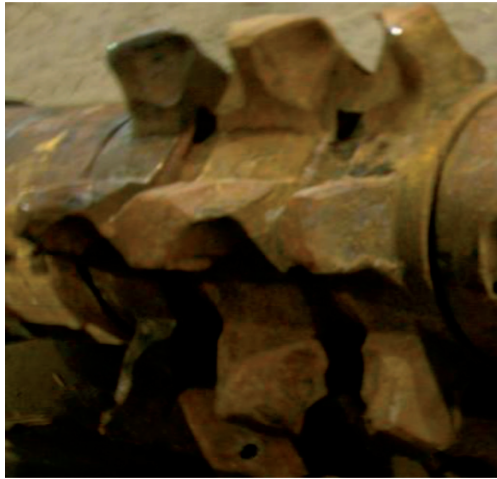
Fig. 1. A sample view of a damaged chain wheel operated in the conditions of combined action of destructive processes
