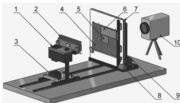
Fig. 2. Scheme of the testing station; 1 - temperature control unit, 2 - infrared radiator, 3 - relay with safety device, 4 - stationary shield, 5 - specimen, 6 - moveable shield, 7 - temperature barrier, 8 - moveable shield drive, 9 - PLC controller, 10 - IR camera
