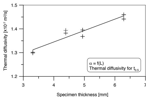
Fig. 15. Effect of specimen thickness on measured values of the thermal diffusivity of neat epoxy resin specimens [15]
