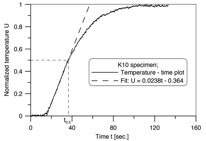
Fig. 11. Normalized temperature versus time at the rear surface for K10 specimen
