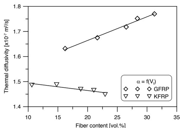
Fig. 13. Comparison of the thermal diffusivity values of GFRP and KFRP composites for different fiber content
